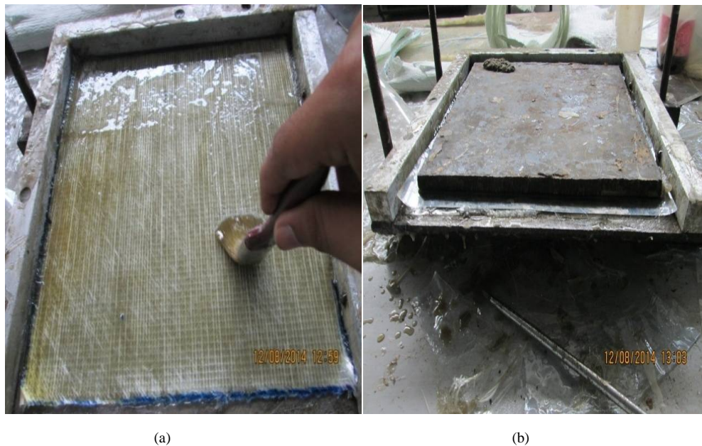
Fig. 2: (a) Hand layup of resin (b) placing the upper mold
